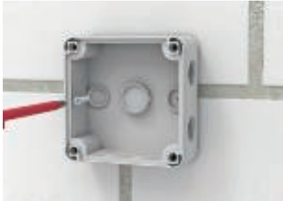
Fastening the B 9/T The fastening holes in the floor area have a soft membrane, which fixes the fastening screws and maintains the protection rating.
