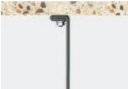
Load 5: Screwed under the ceiling with bolt, belt end doubled, free belt end down Minimum breaking load according to column B
