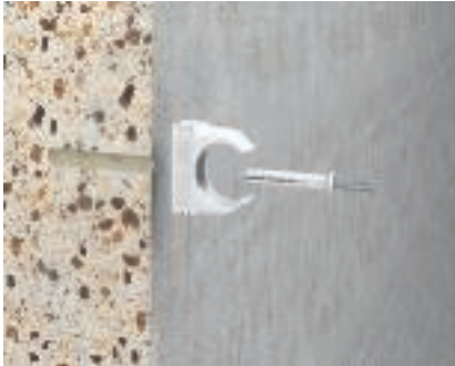
Knock-in anchor 910/SD-Q application Push the knock-in anchor 910/SD-Q into through the fastening hole of the Quick clip.
