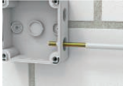
Cable entry The soft membrane of the B 9/T is just pushed through directly with the cable, without any additional tools.
