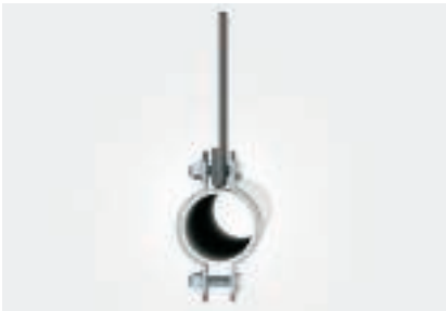
Load 10: Belt end screwed to pipe clamp, belt end doubled Minimum breaking load according to column A
