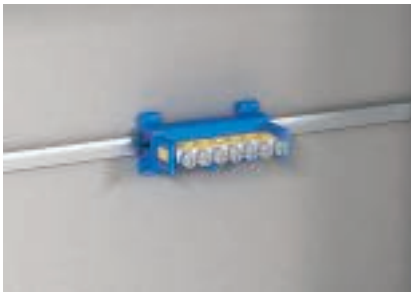
Neutral conductor terminal application Neutral and protective conductor terminals can be snapped onto flat irons, 10 x 2.5 mm, in a lengthwise direction.
