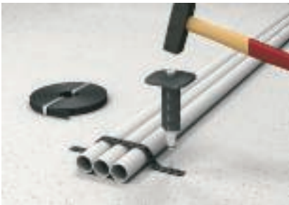
Fastening with installation strip Clips can be quickly bent into any shape using the installation strip, to fasten installation pipes for cable to the floor using OBO anchors, type 903/RB and flatteners.
