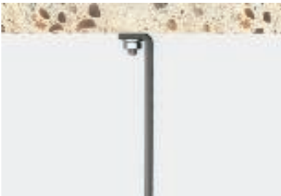
Load 4: Screw under the ceiling with bolt and washer Minimum breaking load according to column C
