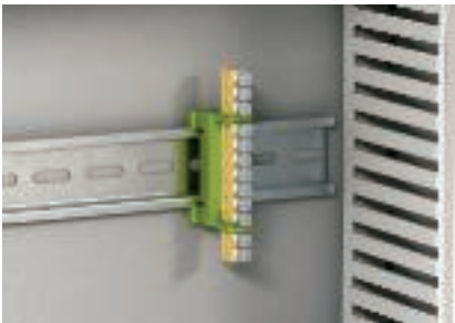
Protective conductor terminal application Neutral and protective conductor terminals can be snapped onto 35 mm hat profile rails in a transverse direction.
