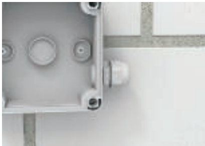
Installation with V-TEC gland The V-TEC cable gland with short connection thread is simply screwed into the available box thread. The soft membrane need not be removed.
