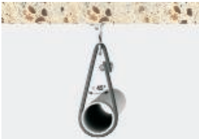
Load 6: Belt wound around flat eyelet and pipe or similar Minimum breaking load according to column 2 x B
