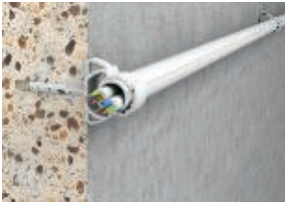
Complete mounting of the Click-snap clip The installation pipe is held by the wings of the clip. The lock provides additional protection, so that the clip cannot open itself by mistake.
