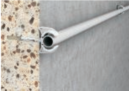
Mounting of Snap clip Prefix the clip in the drill hole using the push-fit anchor. Then attach the pipe and push the pipe with the clip onto the mounting surface.
