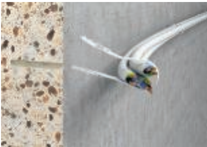
BKS clamp clip application Drill the drill holes, run the BKS clip around the cable and push it into the drill hole.
