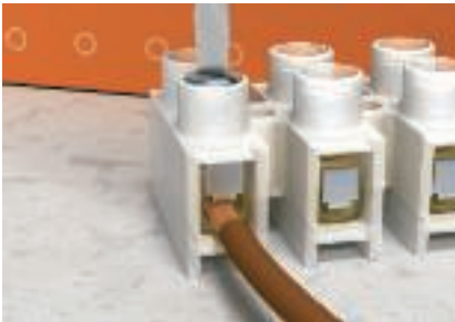
Flexible fine-wire cables The type 74/D means that it is possible to connect fine-wire cables without end sleeves. The wire protection clamp ensures full-surface contacts of the fine copper wires.
