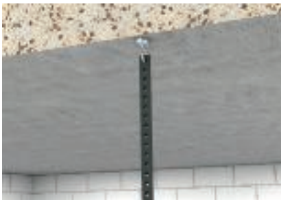
Suspension with installation strip The installation strip can be fastened to the ceiling in many different ways. Here, it is directly suspended from a TS ceiling hook, type 2989, which can be screwed onto an M6 thread.
