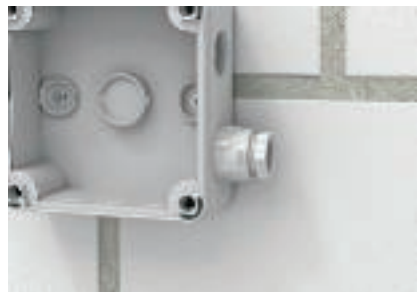
Installation with cone cable gland The conical cable gland with short external thread is screwed into the available box thread. The soft membrane need not be removed.
